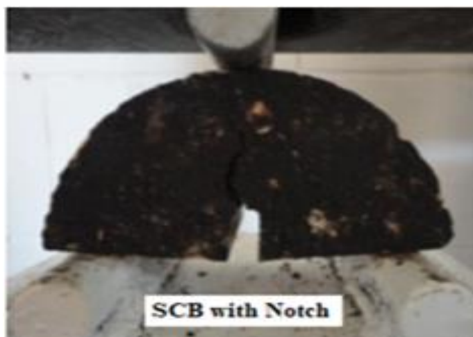
Fig. 3. SCB Specimen with Notch
